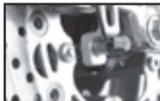
Install the speed sensor on the bracket.
