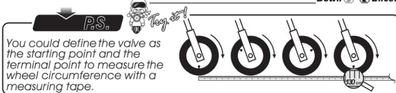
You could define the valve as the starting point and the terminal point to measure the wheel circumference with a measuring tape.
