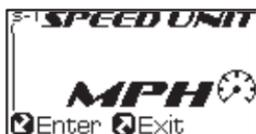
Press button **UP** once (Or the button **Down** 11 times) to select the speed unit setting screen.
