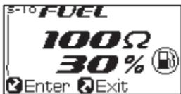
Press button **Enter** to enter the fuel impedance & insufficient fuel warning setting screen.
