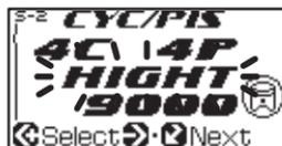
Press button **Enter** to enter the digital needle tachometer range setting
