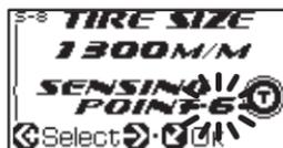
Press button **Enter** to return to the tire size adjustment/ sensor point setting screen.
