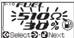
Press button **Enter** to enter the insufficient fuel warning setting screen.
