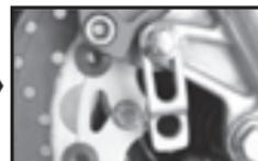
Install the s type sensor bracket.
