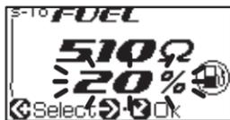
Press button **Enter** to return to the previous fuel sensor impedance setting screen.
