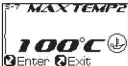
Press button **Enter** to enter the over temperature warning light 2 setting screen.
