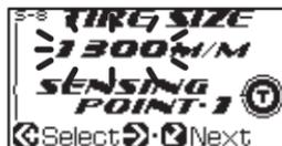
Press button **Enter** to enter the sensor point setting screen.
