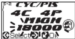
Press button **Enter** to return to strokes/pistons setting screen.
