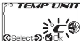
Press button **UP** or **Down** to select the temperature unit.
