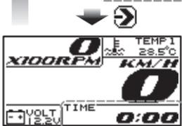
In digital screen: Press button **Down** to switch to the odometer.
