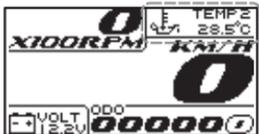
In digital screen: Press button **UP** to switch the oil temperature to the fuel indicator.
