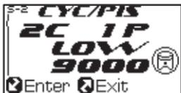
Press button **Enter** to enter strokes/pistons setting screen.
